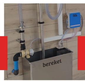
Fix the detergent can to the side of water tank so that only the hot water outlet is placed inside the can
